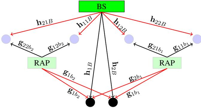
Fig. 2. The channel vectors between the transmitters and receivers are shown in case of limiting the number of primary users, Femto-cells, and number of users in each femto cell to two. For clarity in illustration, the inter-femto cell interference is not depicted. The transmitters are equipped with multiple transmit antennas.
