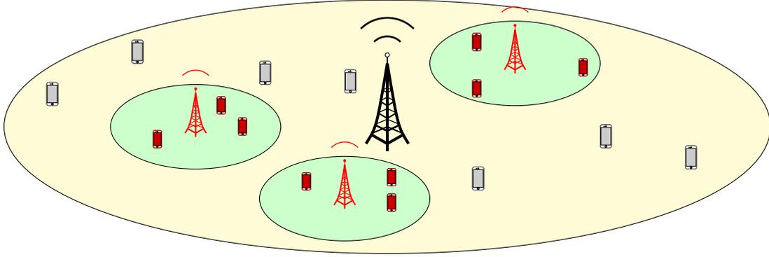
Fig. 1. The primary users in the macro-cell are served by the BS. They demand both information and energy. Furthermore, the secondary users in the femto cells underlay the primary system, i.e., the secondary users are allowed to be active if they fulfil the demands of the primary system. The transmitters are equipped with multiple antennas, while the receivers have single antenna each.
