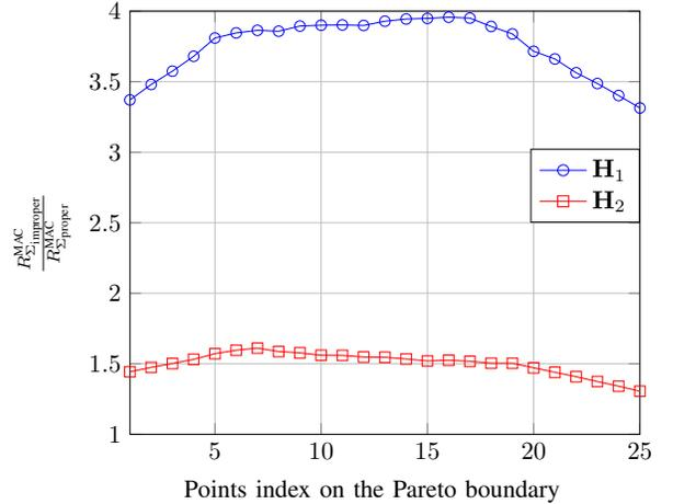
Fig. 4: Improvement in the sum rate of the MAC users by improper Gaussian signaling for  $\alpha_3 = 0.5$ .
