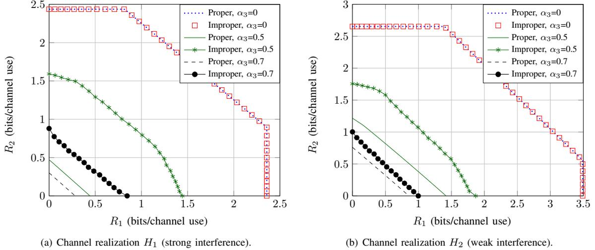
Fig. 3: Comparison of improper and proper signaling at unit maximum transmit power and unit noise variance. The achievable rate region is depicted for the channel realizations  $H_1$  and  $H_2$  corresponding to strong and weak interference, respectively.  $\alpha_3$  is the target rate ratio of the P2P user.
