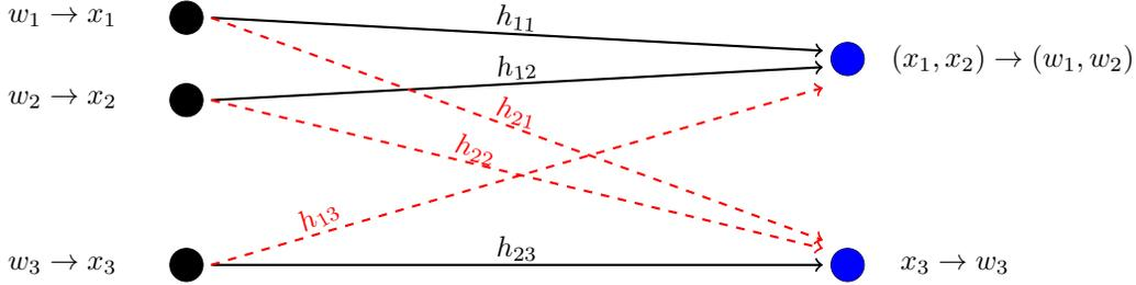
Fig. 2: A Partial Interference Multiple Access Channel (PIMAC). The transmit signals  $x_j$  are a function of the messages  $w_j$  which are the realizations from the Gaussian codebook.
