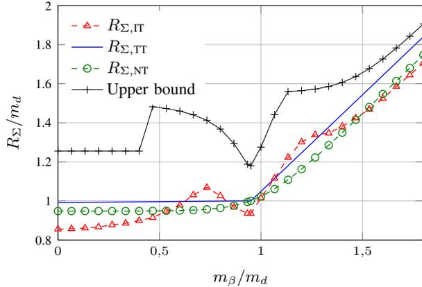
Fig. 2: Normalized achievable sum-rate as a function of  $m_\beta$  for a PIMAC with  $h_d = 1$ ,  $P = 40$  dB,  $m_\alpha = 0.45m_d$  and  $m_c = 0.5m_d$ .
