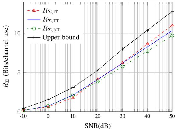
Fig. 3: Achievable sum-rate versus SNR for a PIMAC with  $h_d = 1$ ,  $m_\alpha = 0.45m_d$ ,  $m_c = 0.5m_d$ , and  $m_\beta = 1.2m_d$ .
