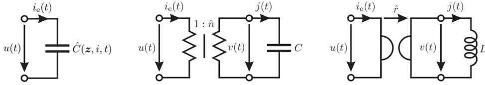
Figure 10: Memcapacitive one-port (left), corresponding electrical representation of a lossless memcapacitive system with a memtransformer (middle), and the dual circuit including a memgyrator (right)
