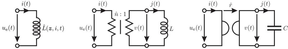
Figure 5: Meminductive one-port (left), corresponding electrical representation of a lossless meminductive system with a memtransformer (middle), and the dual circuit including a memgyrator (right)
