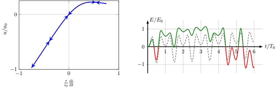
Figure 8: Hysteresis of the meminductive system based on a differential definition (left) and the stored energy within the device (right) for an excitation without (gray-dashed) and with offset (colored). Normalization values are  $u_0 = 3,2$  mV,  $i_0 = 420$  mA,  $\tau = 1$  s,  $E_0 = 80$  nJ, and  $T_0 = 100$  ms.
