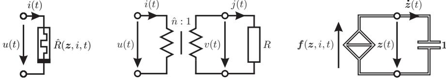
Figure 1: Electrical representation of an  $n$ th-order  $i$ -controlled memristive system. Memristive one-port (left), equivalent circuit with memtransformer (middle), and electrical interpretation of the memory (right).
