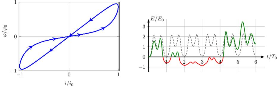
Figure 7: Hysteresis of the meminductive system based on a static definition (left) and the stored energy within the device (right) for an excitation without (gray-dashed) and with offset (colored). Normalization values are  $\varphi_0 = 45 \mu\text{Wb}$ ,  $i_0 = 5 \text{ mA}$ ,  $E_0 = 80 \text{ nJ}$ , and  $T_0 = 100 \text{ ms}$ .
