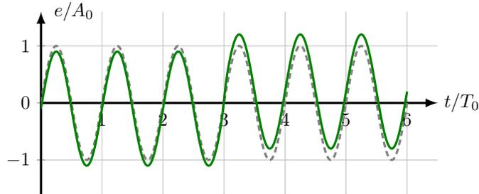
Figure 4: Two excitation signals used in the simulations. On the one hand the sinusoidal excitation without offset (gray-dashed) and on the other hand the sinusoidal signal with negative and positive offset (green). Inserted parameters values are  $A_0 = 0,5$  V,  $A_1 = -0,15$  V,  $A_2 = 0,1$  V,  $k = 100$  Hz, and  $T_0 = 100$  ms.
