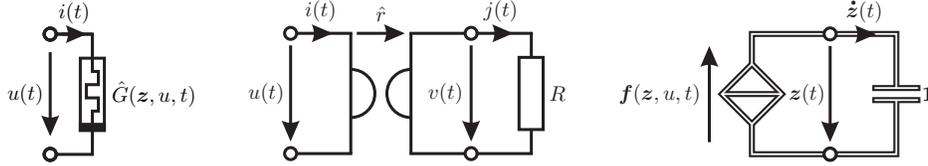
Figure 2: Electrical representation of an  $n$ th-order  $u$ -controlled memductive system. Memductive one-port (left), equivalent circuit with memgyrator (middle), and electrical interpretation of the memory (right).
