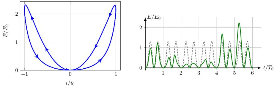
Figure 6: Hysteresis of the meminductive system based on an energetic definition (left) and the stored energy within the device (right) for an excitation without (gray-dashed) and with offset (green). Normalization values are  $E_0 = 0,45$  nJ,  $i_0 = 5$  mA, and  $T_0 = 100$  ms.
