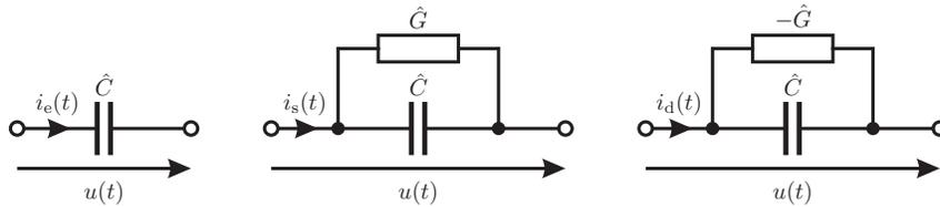
Figure 11: Electrical representation of an energetic (left), static (center) and differential (right) memcapacitive system
