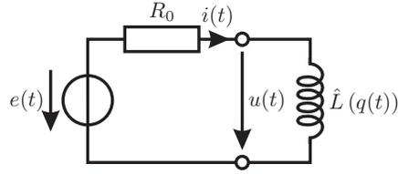
Figure 3: Electrical circuit representing the simulation scenario with internal source resistance  $R_0 = 100\Omega$ .
