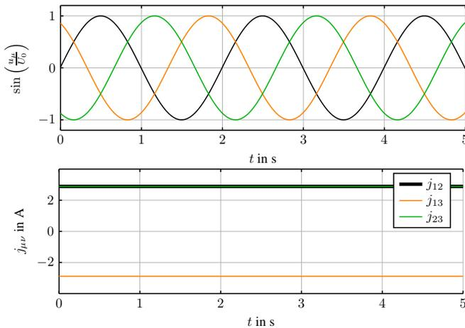
Fig. 7. The three oscillators of Fig. 5 in a zero sum configuration (top). As stated above, the interconnection network in this scenario is internally active while remaining externally passive, as can be seen from not all currents  $j_{\mu\nu}$  being positive (bottom).
