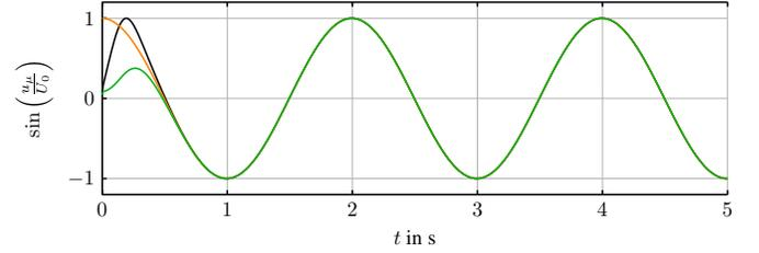
Fig. 8. Two oscillators in an anti-phase configuration with a third oscillator ensuring the transitioning to complete synchronization. This oscillator can be seen as a complete synchronization enabling relays oscillator.
