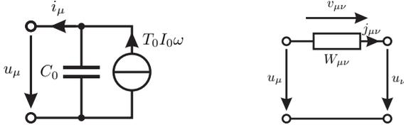
Fig. 1. Integrator circuit with the underlying differential equation (2) (left) and a resistive coupling element to describe one summand of (3), i.e. the input signal of integrator  $\mu$  from integrator  $\nu$  (right).
