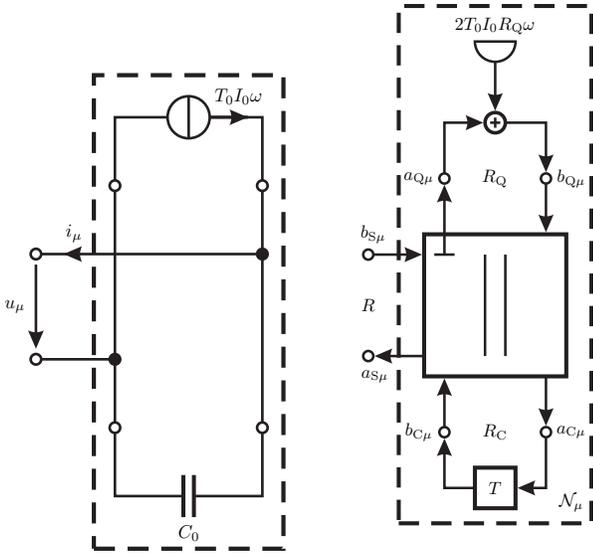
Fig. 4. Integrator circuit described by (2) (left) and its wave digital representation (right).
