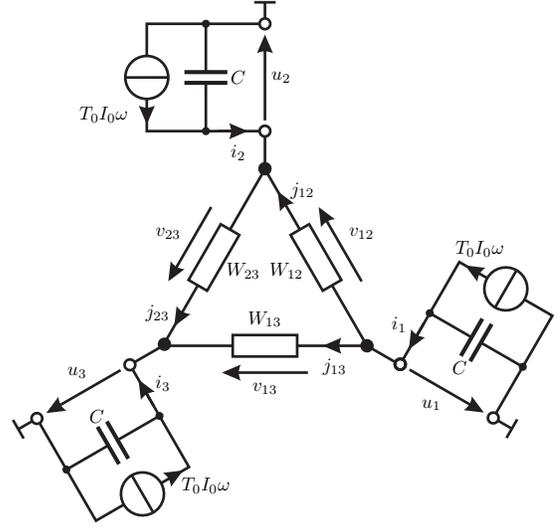
Fig. 2. Complete setup of a system consisting of  $n = 3$  Kuramoto oscillators.
