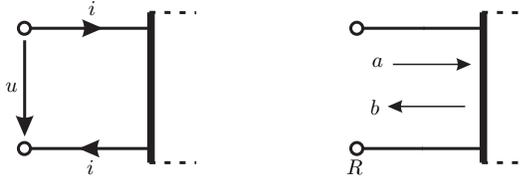
Fig. 3. Definition of a port with current  $i$ , voltage  $u$ , incident wave  $a$ , reflected wave  $b$  and port resistance  $R$ .
