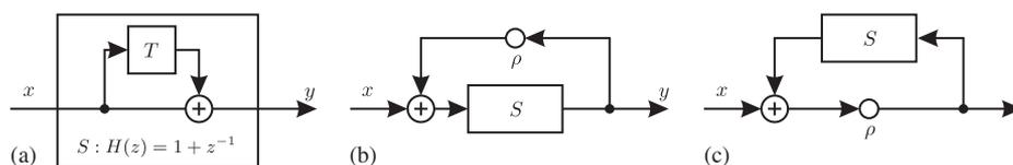
Figure 1. (a) FIR-filter (asymptotically stable) and (b), (c) unstable due to feedback even for  $0.5 < \rho \leq 1$ .
