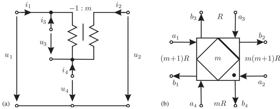
Figure 7. (a) Differential transformer and (b) differential adaptor.
