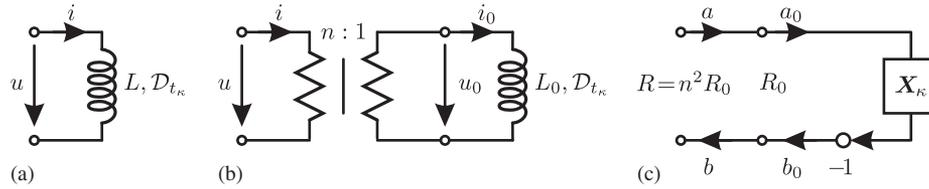
Figure 8. (a) General inductance; (b) decomposition into a transformer with variant turns ratio  $n$  and a constant inductance; and (c) wave digital realization using the trapezoidal rule, expressed in original coordinates.
