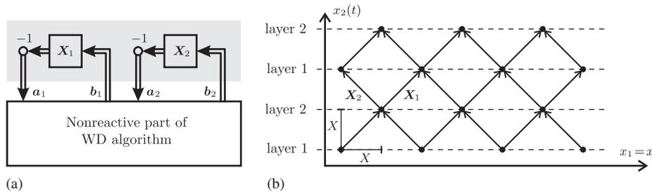
Figure 11. (a) Abstract view of the WD algorithm using the trapezoidal rule and (b) resulting space-time computation scheme.
