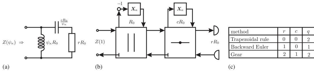
Figure 9. Approximation of an inductance: Passive 1-step ( $c = 0$ ) or 2-step ( $c > 0$ ) method,  $r \geq 0$ . (a) Reference circuit; (b) wave digital algorithm; and (c) well-known methods with consistency order  $q$ .
