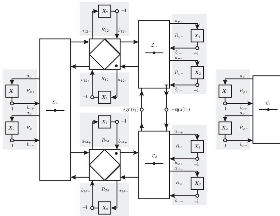
Figure 10. Wave digital algorithm for the fluid dynamic equations.
