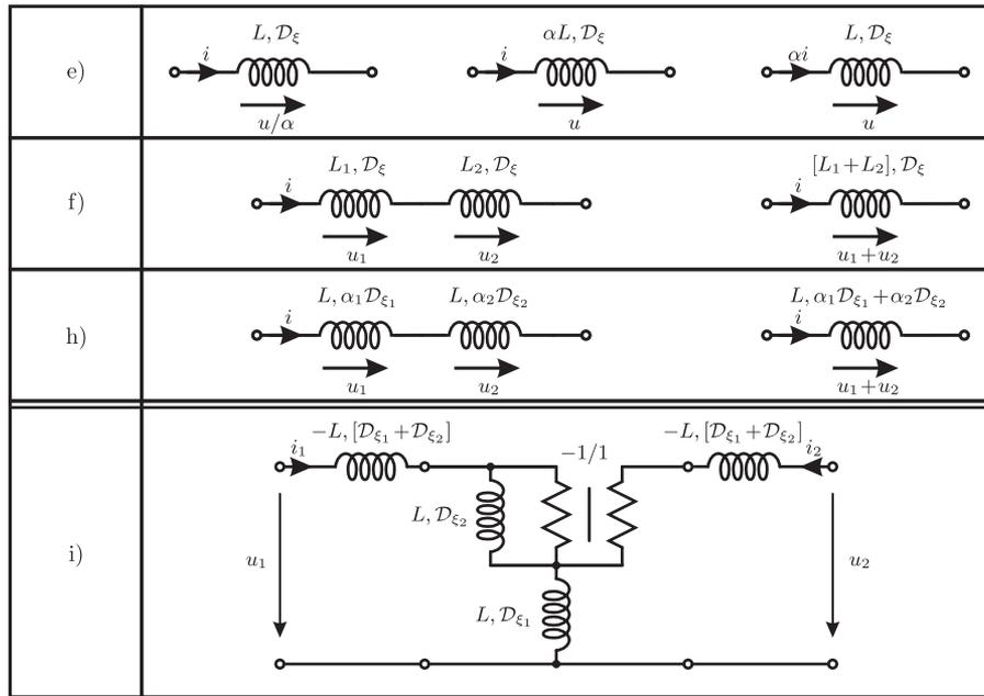
Figure 3. Electrical interpretations for expressions involving the differential operator  $\mathcal{D}$ .
