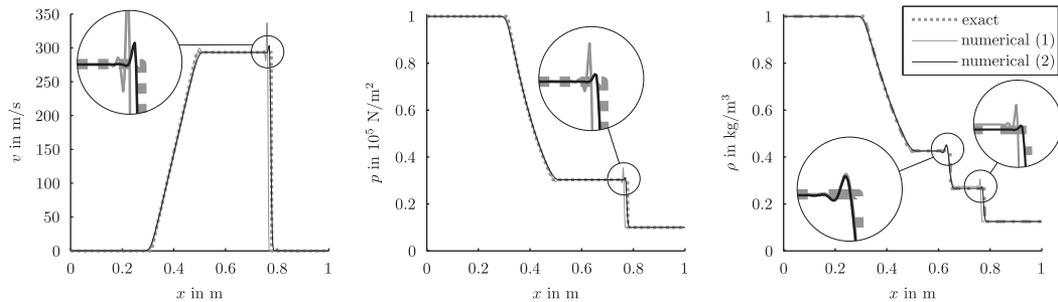
Figure 16. Simulation results using the Gear method, with  $\eta = 0$  (1) and  $\eta = 10^{-1} \text{Ns m}^{-2}$  (2), respectively.
