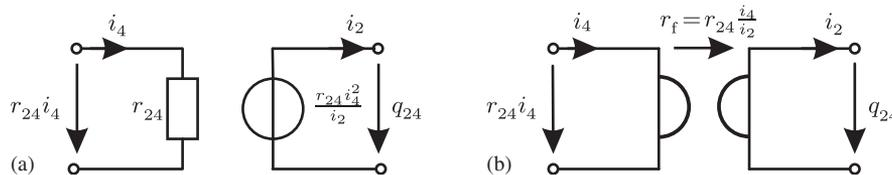
Figure 5. Realization of the friction terms: (a) with resistance and source and (b) internally lossless.
