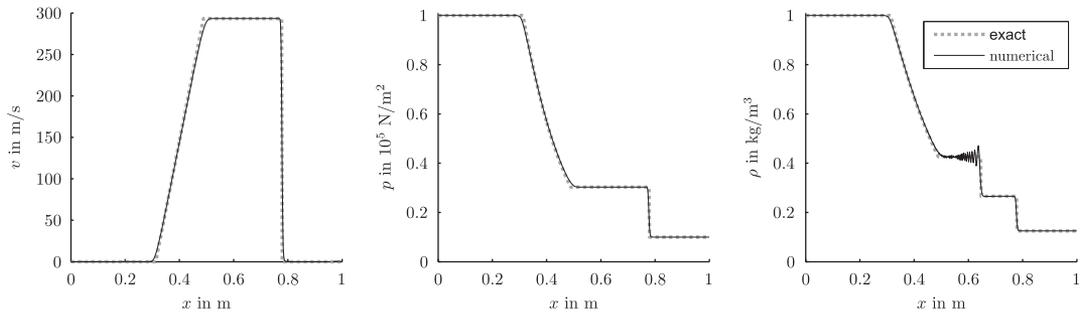
Figure 15. Simulation results using the trapezoidal rule, with  $\eta = 10^{-1} \text{Ns m}^{-2}$ .
