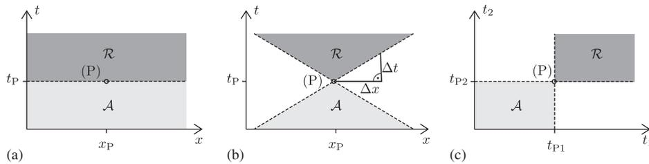
Figure 4. (a) Physical causality; (b) physical causality and finite propagation speed  $v_1 = \Delta x/\Delta t$  (which is assumed to be constant in the diagram for simplicity); and (c) multidimensional causality.
