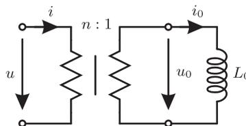
Figure 2. Representation of a general inductance as a composition of an ideal transformer and a constant inductance.
