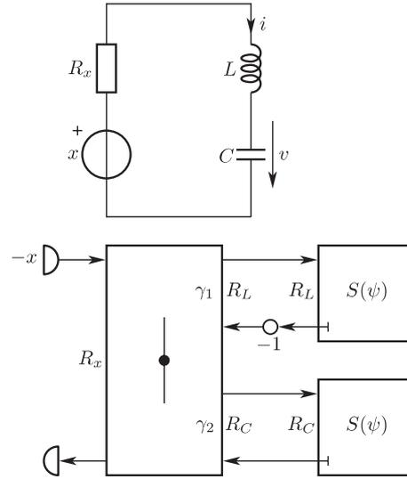
**Fig. 1.** KIRCHHOFF network and its discrete-time equivalent after application of a linear multistep method. Port resistances are  $R_x$ ,  $R_C = Z(1)T/[2C]$ , and  $R_L = 2L/[Z(1)T]$ .
