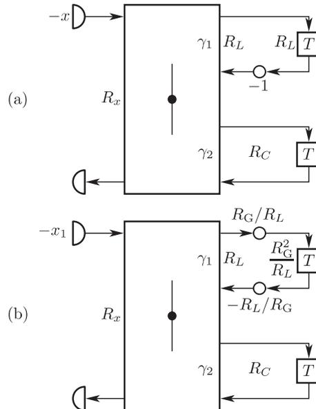
**Fig. 4.** Discrete-time equivalent to the circuit in Fig. 1 after application of the trapezoidal rule and the one in Fig. 2 after application of the GAUSS method.
