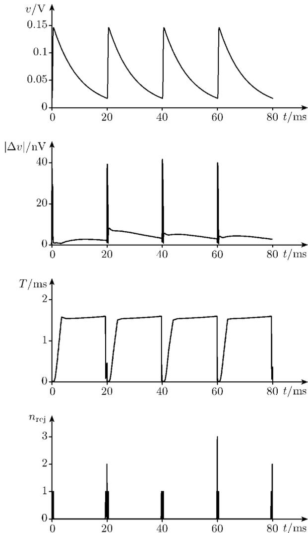
**Fig. 7.** Simulation results for the circuit in Figs. 1 and 2: voltage  $v$  across the capacitance, its deviation  $|\Delta v|$  from the exact solution given in Fig. 6, step-size  $T$  and number  $n_{\text{rej}}$  of rejected step-sizes.
