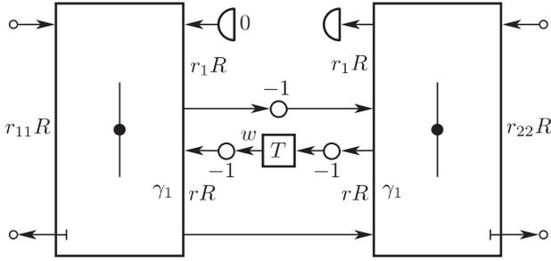
**Fig. 3.** Wave digital realization of the characteristic two-port for a passive 2-stage RUNGE-KUTTA method.
