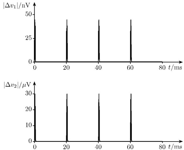
**Fig. 8.** Simulation errors for the voltage across the capacitance obtained with fixed step-sizes  $T_1 = 1/80\,000$  s and  $T_2 = 1/13\,000$  s.
