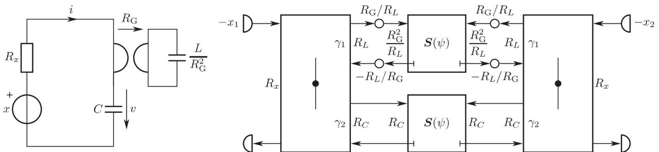
**Fig. 2.** KIRCHHOFF network equivalent to the one in Fig. 1 and its discrete-time representation after application of a two-stage RUNGE-KUTTA method. There holds  $x_1(t_k) = x(t_k + k_1 T)$  and  $x_2(t_k) = x(t_k + k_2 T)$  as well as  $R_C = Z_{11}(1)T/[2C]$  and  $R_L = 2L/[Z_{11}(1)T]$ .
