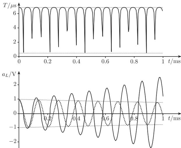
**Fig. 5.** Wave quantity  $a_L$  in the structure in Fig. 4(a) (solid line) and the one in Fig. 4(b) (dashed line) for varying values  $T$ .
