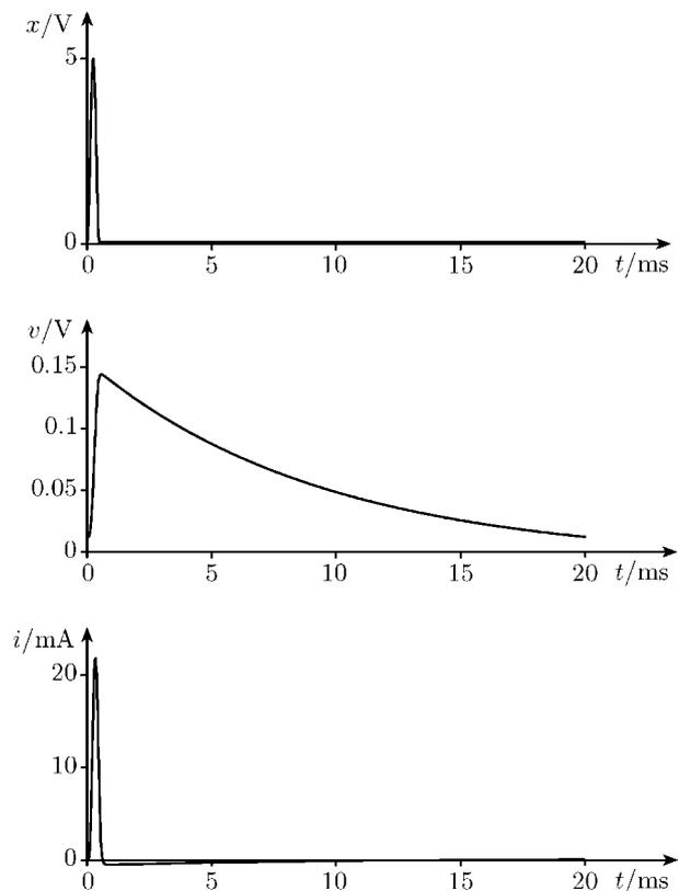
**Fig. 6.** One period of input signal, voltage across capacitance, and current through inductance for the network shown in Fig. 1.
