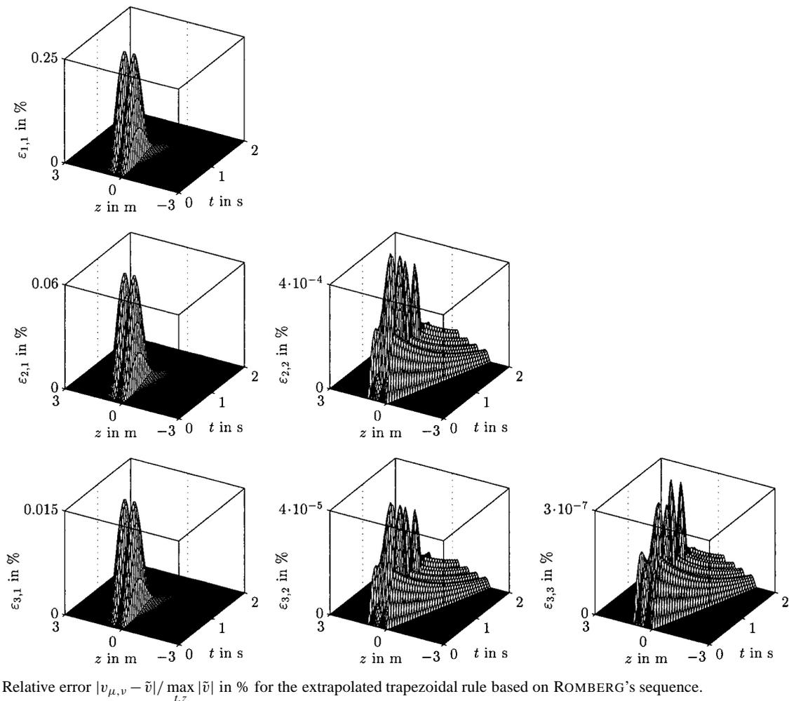
**Fig. 14.** Relative error  $|v_{\mu,v} - \tilde{v}| / \max_{t,z} |\tilde{v}|$  in % for the extrapolated trapezoidal rule based on ROMBERG's sequence.
