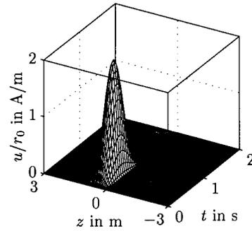
Fig. 12. Product of two  $\sin^2$ -pulses used for the excitation of the telegraphists equations.
