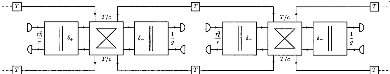
Fig. 11. Uncoiled wave digital structure corresponding to Fig. 10.
