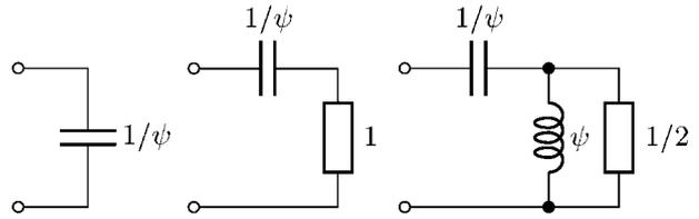
**Fig. 1.** Characteristic impedances for some passive linear multistep methods. From left to right: trapezoidal rule, implicit EULER and GEAR's procedure.
