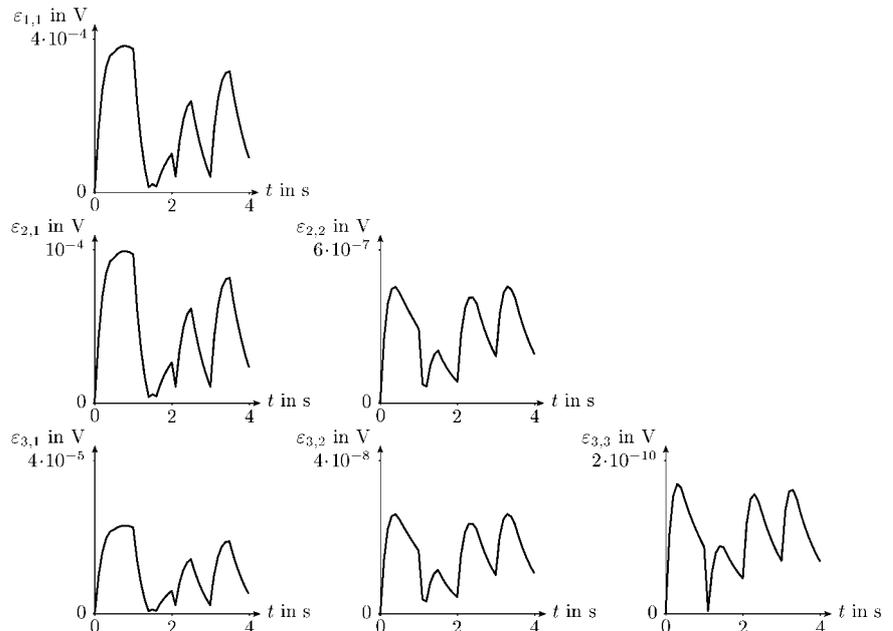
**Fig. 8.** Deviation  $\varepsilon_{\mu,\nu} := |v_{\mu,\nu} - \tilde{v}|$  for the extrapolated trapezoidal rule based on ROMBERG's sequence.
