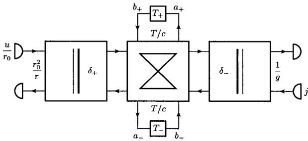
Fig. 10. Wave digital structure corresponding to Figure 9.
