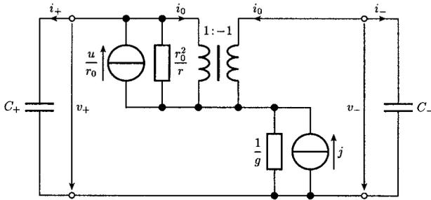
Fig. 9. Circuit representation of the telegraphists equations (39).
