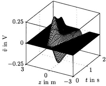
**Fig. 13.** Exact solution of the telegraphists equations for the excitation given in Fig. 12.
