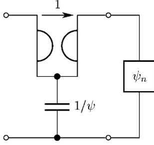
**Fig. 2.** Concretely lossless KIRCHHOFF network with (normalized) impedance  $\psi_{n+1}$ .
