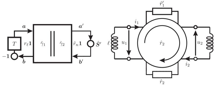
Figure 9. Left: A wave digital structure for a state-space model with a real eigenvalue of algebraic multiplicity  $n$  and geometric multiplicity 1. Right: The corresponding electrical circuit for two states.
