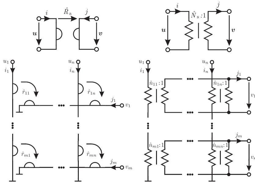
Figure 1. Top: Symbols of a multiport gyrator (left) and a multiport transformer (right). Bottom: Internally passive circuits for a multiport gyrator (left) and a multiport transformer (right).
