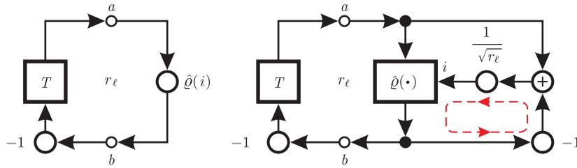
Figure 10. Wave digital model of a lossless oscillator (left), possessing a latent algebraic loop (right).
