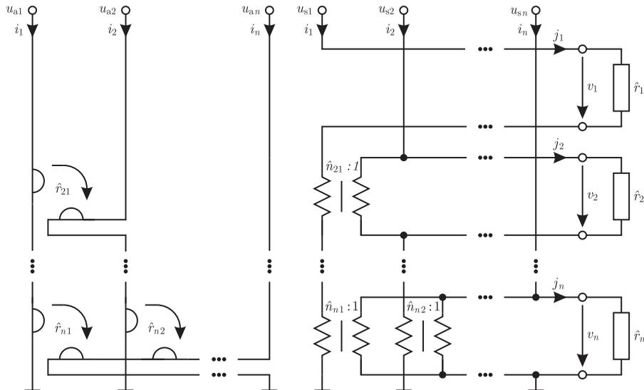
Figure 2. Canonical internally passive circuits for an antimetric and a symmetric multiport resistance, respectively.
