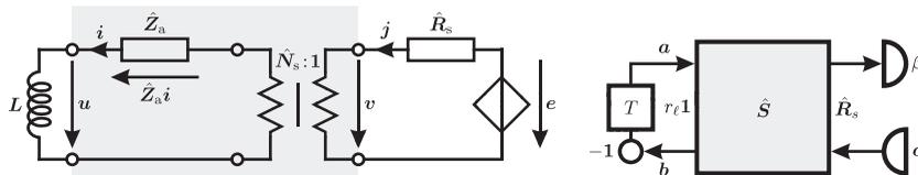
Figure 4. Electrical circuit of a state-space model and its draft for a wave digital modeling.
