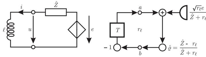
Figure 6. An electrical circuit and its wave digital realization for a scalar state-space model.
