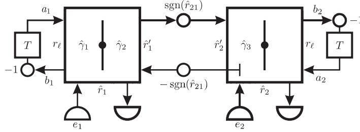
Figure 8. A wave digital structure for a real state-space model with two states and  $\hat{n}_{21} = 0$ .
