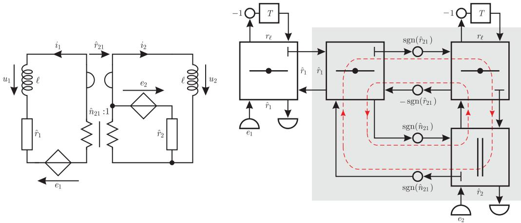
Figure 5. Left: Electrical circuit of a state-space model with two states. Right: Corresponding wave digital structure containing delay-free directed loops.
